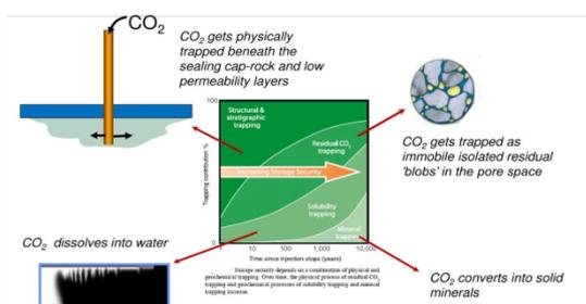
Fig1. A sketch of key processes governed by capillary trapping after CO<sub>2</sub> injection has ceased at a storage site. Plume migration is limited by the trapping as large fractions of the plume are immobilised.
