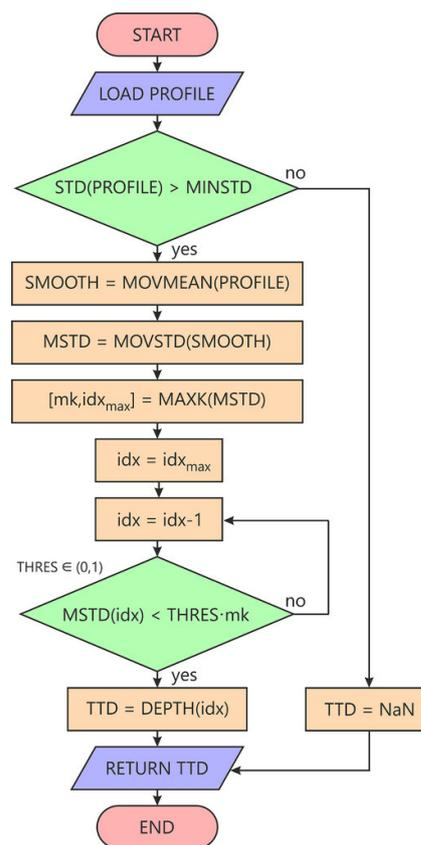
Figure 1. The flow diagram of the "MovSTD" algorithm, source: Janecki et al. (2022).
