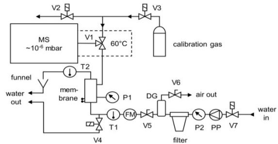
Figure 1. Schematic Diagram of the GE-MIMS.
