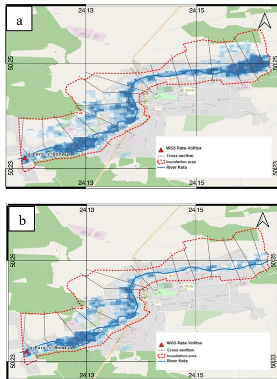
Figure 1. Flooding zone during the passage of spring flood (a) and rain flood (b) in the area of the WGS Rata River - Volitsa according to the calculated hydrograph (Q1%)
