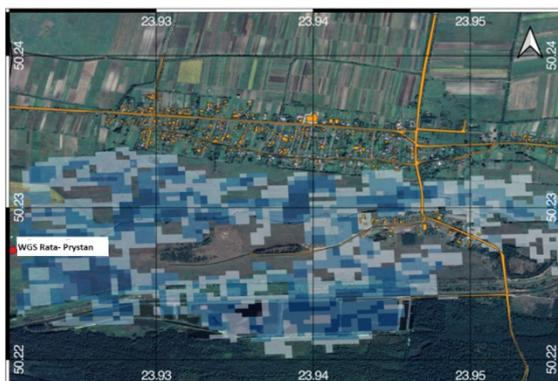
Figure 3. Flooding zone during the passage of spring flood in the area of the WGS Rata River - Prystan according to the calculated hydrograph (Q1%) in the absence of observations of the runoff
