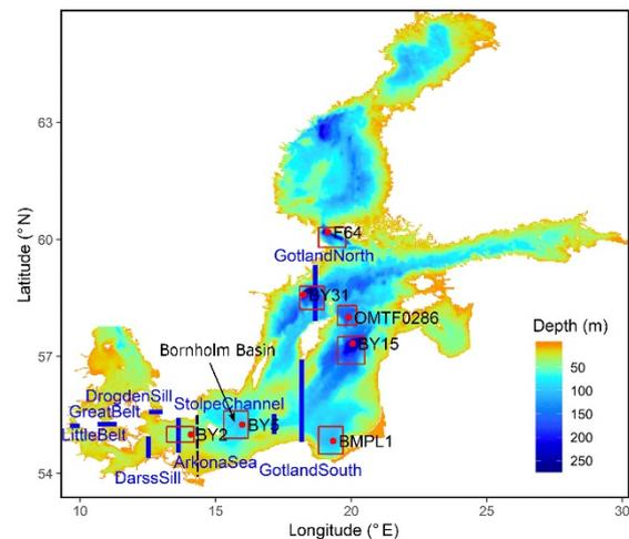
(taken from Radtke et al. (2020) and modified). Blue lines denote transects for salt transport calculation. The thin dashed line indicates the eastern boundary of the Arkona Basin for the salt content calculations (S17). Red squares show areas around selected stations from which observational data was taken for the model validation.
