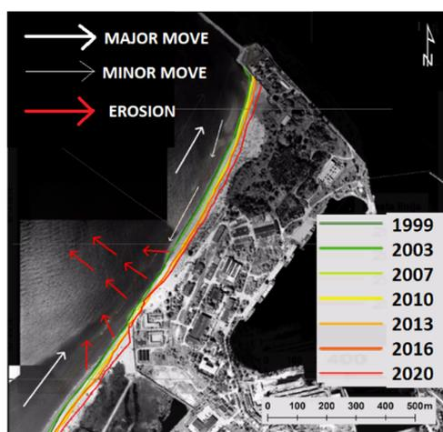
Figure 3. Shoreline changes (coloured lines) and scheme of the sediment transport after the rock revetment was built ca 650 m south from the breakwater.
