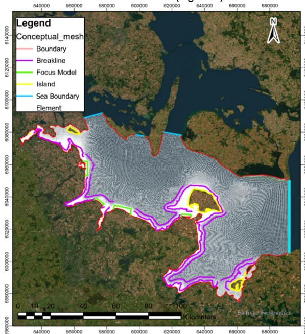
Figure 1. Domain and unstructured computational mesh of the coupled regional hydrodynamic model
