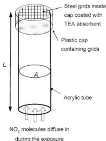
Figure 3. Nitrogen dioxide (NO<sub>2</sub>) Palmes passive diffusion tubes.
