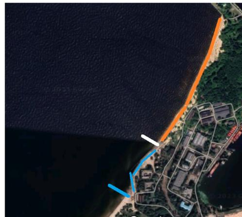
Figure 4. Scheme of the proposed solution. First step: jetty (white). The second: beach nourishment with sand (orange). The third: another jetty (blue). The lengths are schematic and need to be determined in the second part if this option is chosen.
