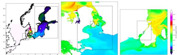
Figure 1. Inserting high resolution domains with two-way nesting. Left: North Sea-Baltic Sea, middle – Øresund domain, right – Copenhagen domain
