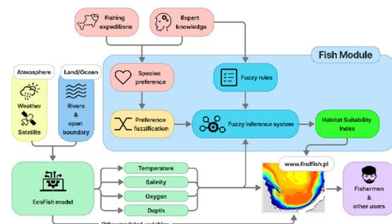
Figure 1. The general outline of the Fish Module algorithm along with the interdependencies between the elements implemented in the FindFISH project. Source: Janecki & Dzierzbicka-Głowacka (2024, In Press).
